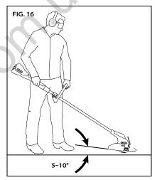
Push the trimmer head slowly from the side into the grass or weeds to be cut, and move the trimmer head back and forth so that the end of the trimmer line contacts the material to be cut.
