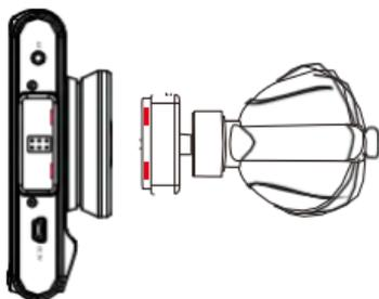
Holder base one side have 2 gaps must be fit into camera body 2 clips
