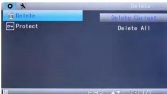
In playback mode, press Menu button, select “Protect”, you will have protect lock options (“lock one” to protect the selected file, “lock all” to protect all the files on the memory card) and protect unlock options (“unlock one” to unlock the selected files, “unlock all” to unlock all the protected files on the memory card).
