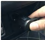
Car Charger get power from car lighter
