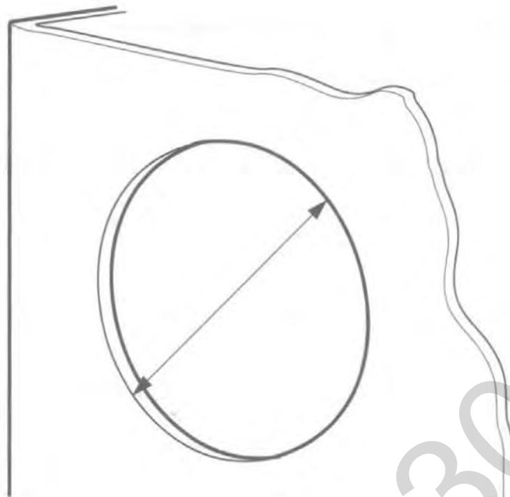
Make the mounting hole as follows. The mounting hole cut dimensions is 50 mm (2 in.)
