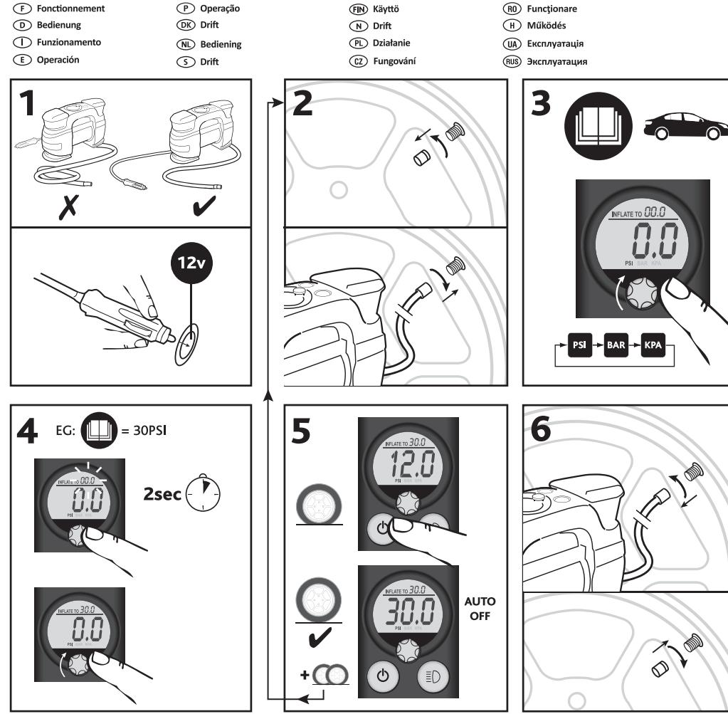
**NOTE:** The gauge on this compressor is for guidance only. Check pressure with a known accurate gauge. The compressor can be used without the engine running but this will drain the power from the battery.
