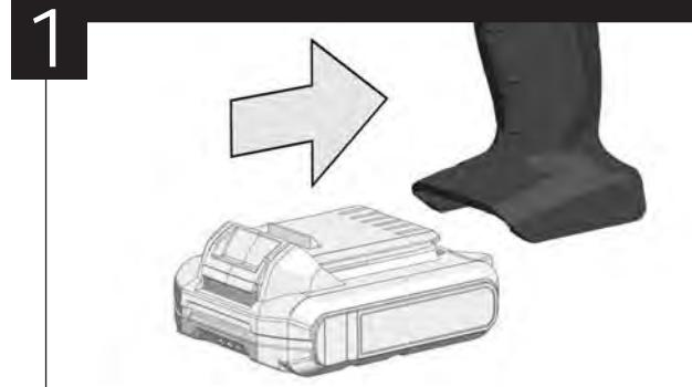
Remove the battery pack before starting any work on the machine.
