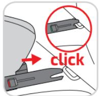
The ISOFIX mounting points are located between the seat and the backrest of the car seat.
