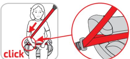
Place the MaxiFix PLUS on the car seat, set your child in the Booster and secure your child with the lap (O) and diagonal belts (N) of the three-point-vehicle-belt.
