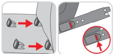
Before placing the MaxiFix PLUS on the car seat, fasten if necessary in your vehicle the two supplied mounting aids (IH) to the ISOFIX anchors (IA). The ISOFIX mounting points are located between the seat and the backrest of the car seat.
