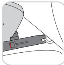
Lay the top tether (TT) over the child car seat. Place the HEYNER® MultiRelax AERO Fix on the car seat in the driving direction. Check the safety indicators on the ISOFIX arms (IM). Both of them have to be red. If the safety indicators are green, you have to unlock the ISOFIX arms (IM) before you connect them. You can do this by pulling back the ISOFIX release button (IT) until a <<click>> sound is clearly heard.
