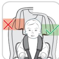
In order to adjust the height of the headrest (A) to the size of your child, grasp the headrest from above and pull the adjustment lever (H) up.
