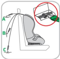
This one you can find by means of the instruction manual of your car. Hook on the top tether and pull the belt tight.
