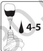
**NOTE: Before the first use of the tool, apply 4-5 droplets of oil to the inlet opening before connecting the hose.**
