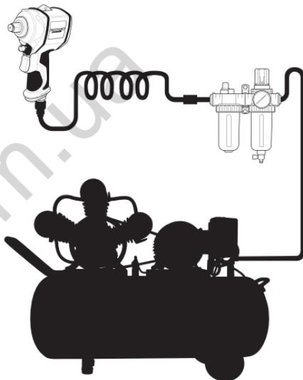
All control elements, connecting lines and hoses should be intended for the necessary pressure and the air flow rate. Do not allow the narrowing of feeding lines, for example, as a result of cross-clamping, bending, or stretching. Before connecting a hose to the tool, regularly blow the hose with a strong air stream to remove moisture from the hose.
