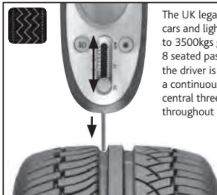
The UK legal minimum tread depth for cars and light trailers (inc caravans) up to 3500kgs gross vehicle weight and or 8 seated passenger vehicles including the driver is a minimum of 1.6mm in a continuous band throughout the central three-quarters of the tread width throughout the whole of the circumference
