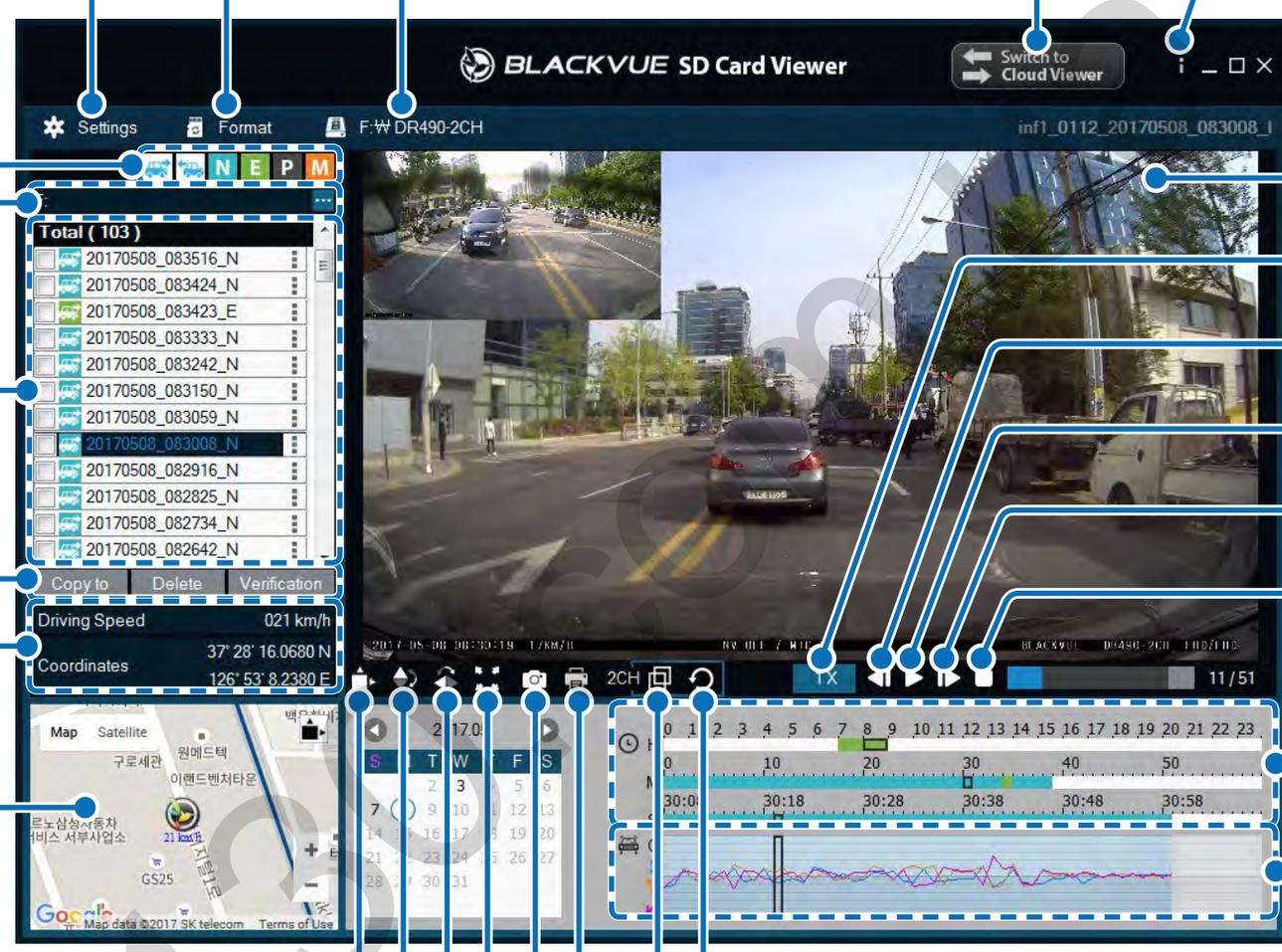
The screenshot shows the main interface of the BLACKVUE SD Card Viewer. It features a central video playback window, a file list on the left, a map at the bottom left, and a playback control bar at the bottom. The interface is annotated with numerous labels in Russian, pointing to specific UI elements and their functions.
