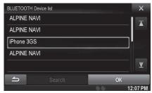
The system starts searching for BLUETOOTH devices. When the search is completed, the BLUETOOTH Device List is displayed.
