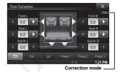
cm/inch: Adjust listening position and distance from each speaker.ms: Adjust time.
