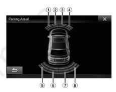
If the parking assist interruption occurs during the camera mode, a small parking assist image will display on the right side of camera screen. Touch the image can see the full screen of parking assist
