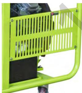
Loosen the protective cover to get access to the battery.
