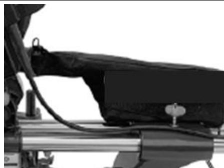
The machine is equipped with a chip bag for sawdust and chips.
