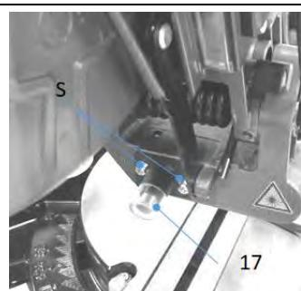
If the laser (17) does not show the correct cutting line any more, you can adjust the laser. Loosen the Phillips screws (S) and adjust the laser by moving it sideways until the laser beam hits the teeth of the saw blade. Tighten both screws (S) again.
