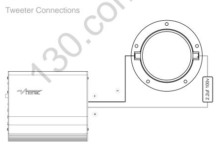
**NOTE :** Unless using an active crossover network, the 2.2uf 100v capacitor must be fitted in order to avoid damage to the tweeter.
