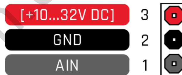
Figure 2 MSP500 socket pinout
