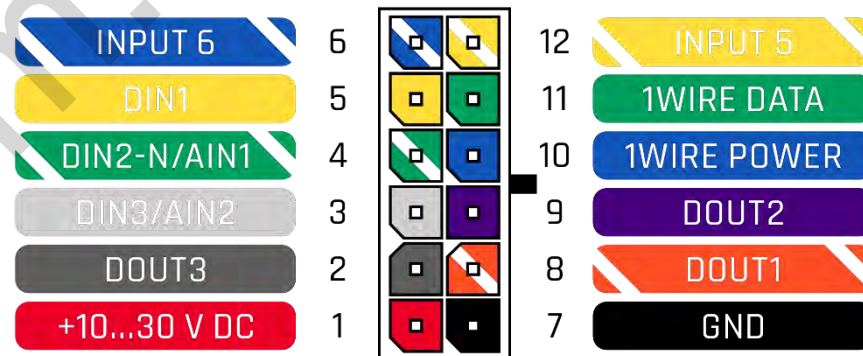
Figure 2 FMU130 2x6 socket pinout
