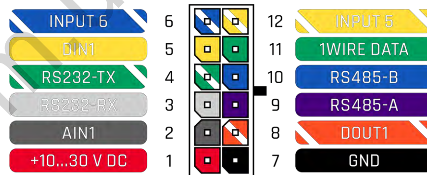
Figure 2 FMB125 2x6 socket pinout
