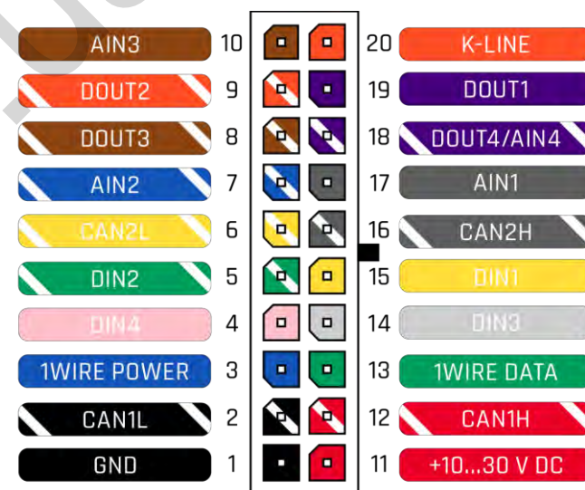
Figure 2 FMC640 pinout
