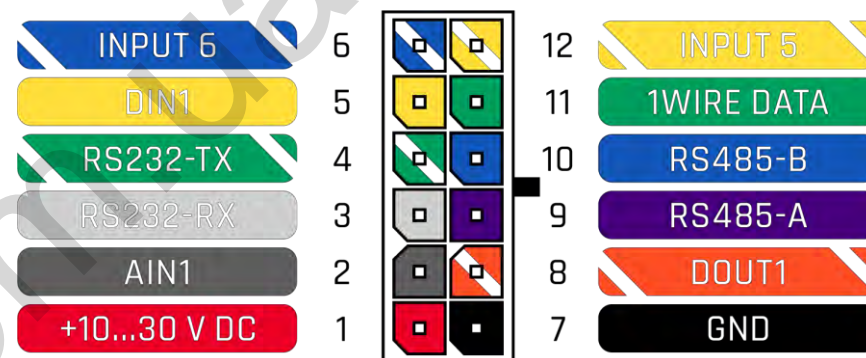
Figure 2 FMC125 2x6 socket pinout
