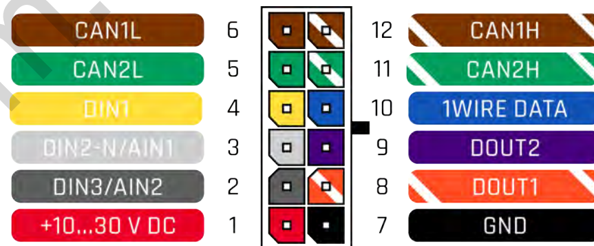
Figure 2 FMB140 2x6 socket pinout
