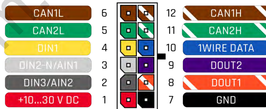
Figure 2 FMB140 2x6 socket pinout
