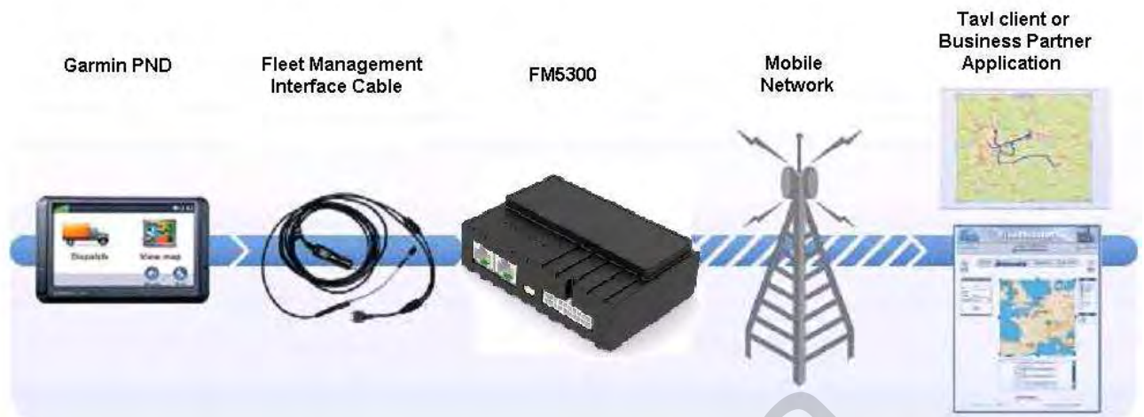
Figure 548 FM53+Garmin operational scheme
