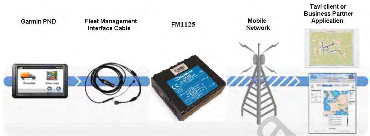
Figure 63 FM1125+Garmin operational scheme
