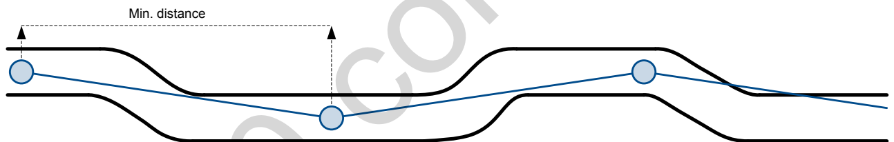
Figure 28 Distance based data acquiring example
