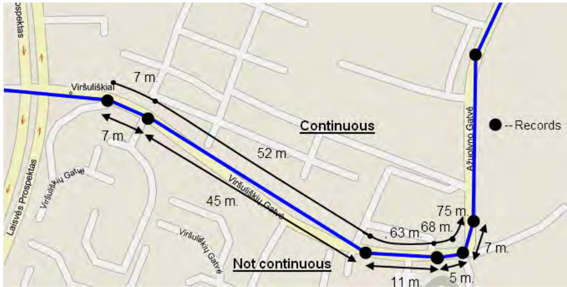
Figure 33 Trip continuous distance counting parameter example
