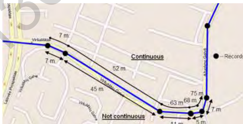
Figure 24 Trip continuous distance counting parameter example
