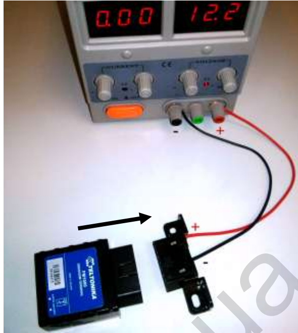
Figure 10 inserting FM1010 to OBD-II connector
