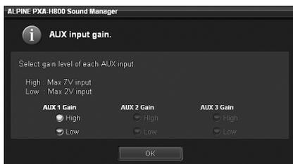
High: When the volume level of the external input is high.
