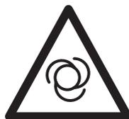
Warning! The unit is equipped with an automatic start control. Keep others away from the work area of the device!
