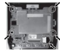
5 Lift up the board, disconnect the connector, and remove the battery.
