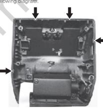
The hooks can be released with a flathead screwdriver.
