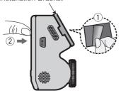
Use extreme care as the double-sided tape on the Installation Bracket in (①) is extremely strong, and it will be difficult to reapply the tape once it has been applied.
