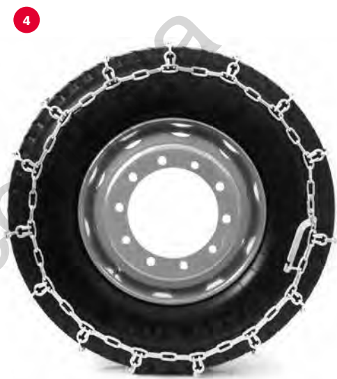
Then tighten the outside chain and close it by means of the tension lever.
