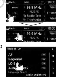
The unit tunes in only to stations with sufficient signal strength. The LO.S indicator lights up.
