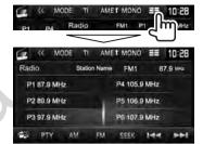
The preset list and the station name for FM Radio Data System (when PS signal is coming in) are displayed.
