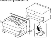
Bend the tabs of the mounting sleeve with a screwdriver or similar utensil and attach it in place.
