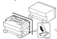
Bend the tabs of the mounting sleeve with a screwdriver or similar utensil and attach it in place.
