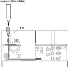
\* Use CA-U1EX for extending the cable if necessary. (Max 500 mA, 5V)
