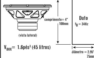
$$V_{\text{BOX}} = 1.6 \text{ pés}^3 (45 \text{ litros})$$
