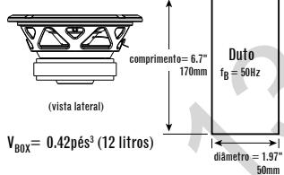
$$V_{\text{BOX}} = 0.42 \text{ pés}^3 (12 \text{ litros})$$
