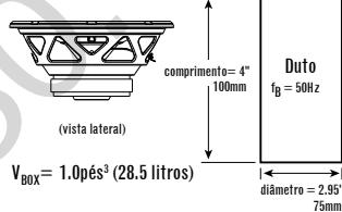
$$V_{\text{BOX}} = 1.0 \text{ pés}^3 (28.5 \text{ litros})$$
