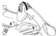
**Air purge:** Press the air purge repeatedly until fuel begins to fill the bulb. The bulb need not be completely filled.
