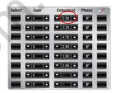
Further detailed adjustments can be edited to either the time alignment list (ms) or to the speaker distance window (cm)
