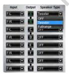
The mentioned information to channel A, B, C and D refer to the speaker output of the GZDSP 4.80AMP. The signal of channel E, F, G and H will be available at the RCA line output (via line out harness).
