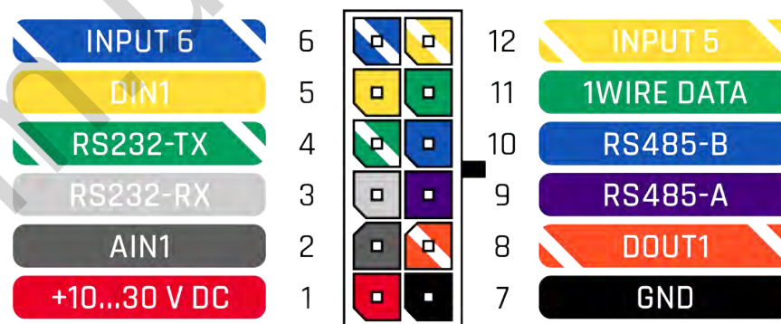
Figure 2 FMB125 2x6 socket pinout
