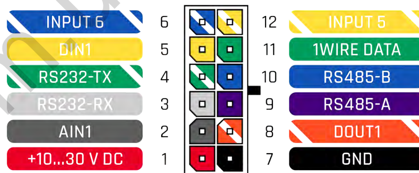
Figure 2 FMB125 2x6 socket pinout
