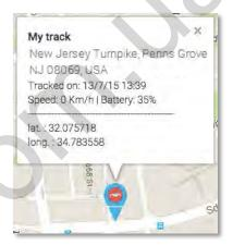
Note: The device location may be based on the cellular network signal (GSM location), in cases where the device cannot receive proper GPS signals from the GPS satellites, for example indoors. This location is not accurate, but rather an approximation of the device location.
