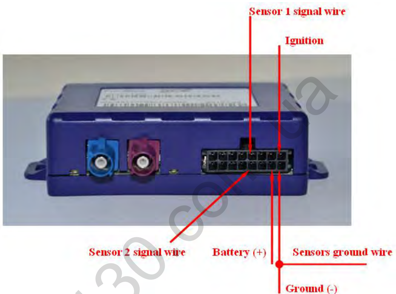
Fig. 4. Two sensors connection to FM blue+ using analog mode.
