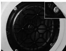
Cutting-out of rivets with a  $\varnothing 5,5/6$ mm metal drill.
