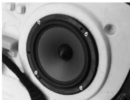
Focal speaker riveting (aluminum 4x16mm rivet).
