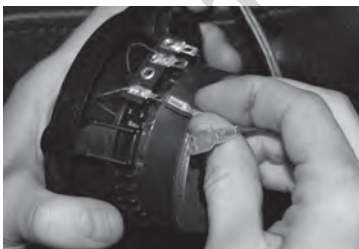
5. IFBMW-S wire connection on the speaker terminal.
