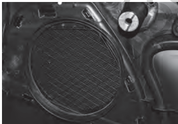
11. Factory speaker grille location. Be careful that the IFBMW-S cone doesn't come in contact with the panel.
