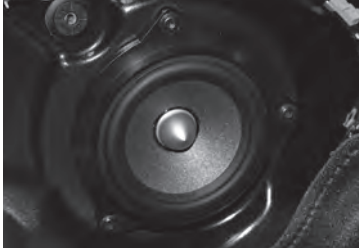
7. IFBMW-S assembled in the door.
