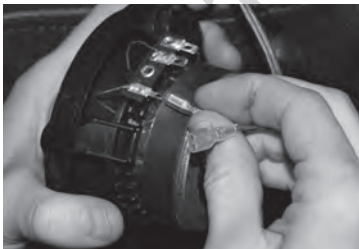
5. IFBMW-S wire connection on the speaker terminal.
