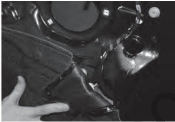
3. Remove the Foam protection to pass the wire inside the door.
