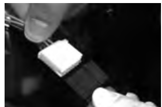
TOYOTA® factory connector plugged in the IS 165TOY tweeter
