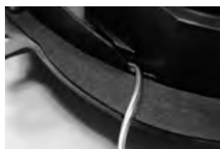
Pass the connector cable in the dedicated space
