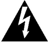
This lightning flash with arrow symbol within an equilateral triangle is intended to alert users that there might be uninsulated dangerous voltage which may cause
