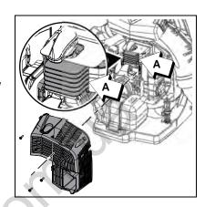
Parts Required: Spark Arrestor Screen
