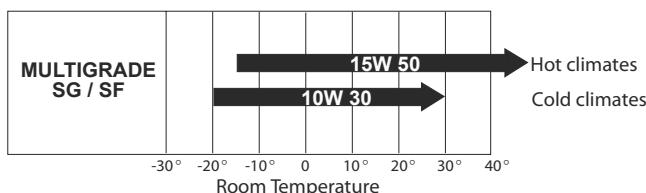
Use detergent oil for four-stroke engines, class API SG or SF (indicated on the oil can) with SAE viscosity suitable for the climate (see table).
