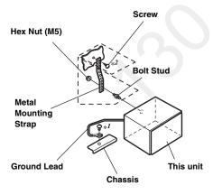
For the screw marked "\*2", use an appropriate screw for the chosen mounting location.
