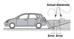
The distance guidance mark represents the distance to a flat road surface. Therefore in the case of an upward slope behind the car, the distance guides are displayed closer to the rear bumper than the actual distance. For example, if there is an obstacle on the upward slope, it may appear farther away than its actual position.
