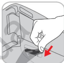
In order to remove the crotch belt, push the belt, together with the metal plate, out of the seat part from bottom to top.
