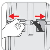
Loosen the belt ends of the harness belts (**G2**) on the back side of the seat part (**ST**) from the belt anchor (**R**).
