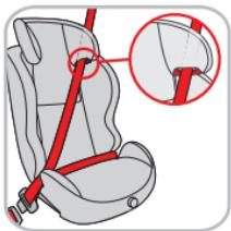
Attention: The belt should not be twisted. To ensure an optimum belt run, the headrest should be adjusted correctly to the child.
