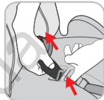
Now you can completely remove the five-point belt system. The central adjustment belt (**G5**) can be stored under the adjuster cover (**F**).
