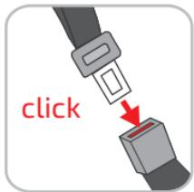
A flat hand should fit snugly between the belts and the body of the child. Adjust belt height adjusters, in case you have them in your car, to the size of the child and to the size of the seat. Check the run of the belts and the height of the support for the head from time to time and adjust them to the growing child.
