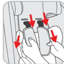
In order to remove the crotch strap, push the belt, together with the metal plate, out of the seat part from bottom to top
