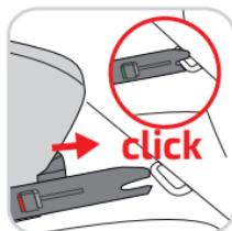
Now release the ISOFIX adjustment button (IE) and make sure that that both clips do not slip back.
