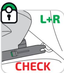
Please check by means of the safety indicators on **BOTH SIDES**, if the seat is connected correctly with both ISOFIX anchors (IA) of the car.
