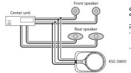
Connect the subwoofer to the front or rear output cords of the center unit.
